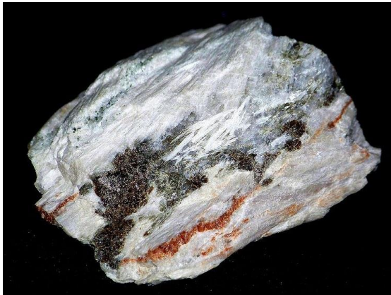
A piece of wollastonite, mixed with other minerals, from a Polish mine. The wollastonite is white, and its fibrous structure can be seen. Photo by Piotr Sosnowski, from Wikipedia. Creative Commons licence.
