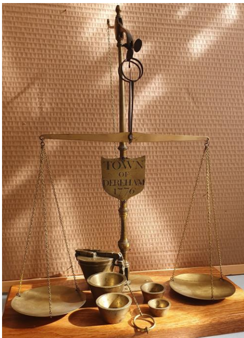
Fig 3. Dereham's town scales of 1776, used to check the honesty of traders' weights. The five comparison weights range from ¼ ounce (7.1g) to 8 ounces (226.4g). On display in Bishop Bonner's Cottage Museum.
