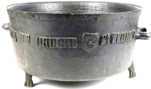
Fig 2 The Bronze Exchequer Standard Winchester Bushel volume measure, distributed in the reign of Henry VII. (Photo ©The Board of Trustees of the Science Museum. Used under a Creative Commons Licence https://collection.sciencemuseumgroup.org.uk/objects/co58279/exchequer-standard-winchester-bushel-measure-winchester-capacity-measure-standards ) Image contrast enhanced.
